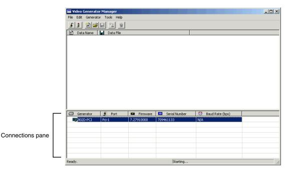
VGM adds the generator to the connections pane. VGM may be connected with multiple generators, but can control only one generator at the same time.
